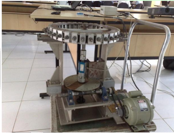
Low Speed Flywheel Mounted on Test Jig.
