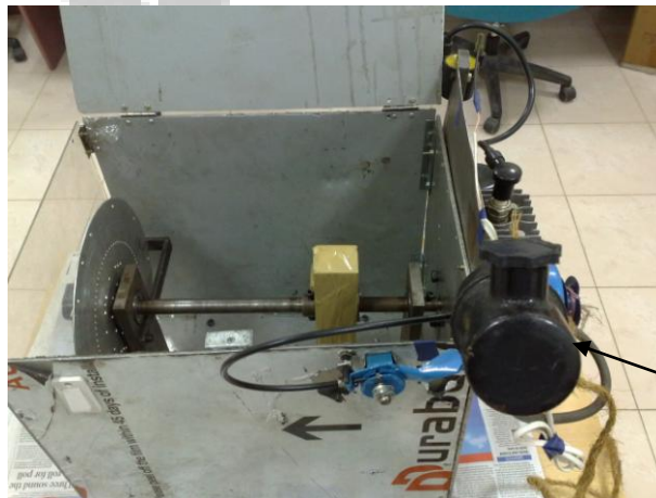
Low Speed Flywheel Mounted on Test Jig.
